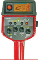
Radio remote control with digital feedback
