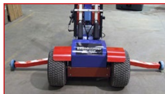
Comes with durable offroad front and rear tyres for added grip over surfaces.
