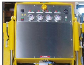
Control panel with quad-circuit vacuum and 90° twin hydraulic tilt cylinder system
