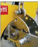
Lowered suspension for installation of transom windows offers a coupling point in the center of the lifter, allowing a reduced distance of the hook.
