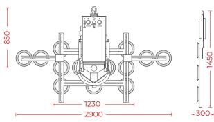
\* The capacity is only 1000kg with extension arms and 14 pads fitted.
